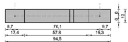
**BALLAST DIMENSIONS AND PANEL HEIGHT FROM THE GROUND - UNIT OF MEASUREMENT cm
